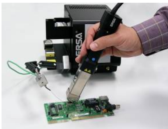
Figure 8: Closed loop temperature of PCB during rework
