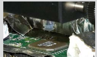
6. Resolder the BGA on the prepared surfaces of the board
