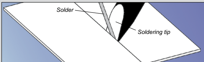
Guiding the soldering iron when soldering a narrow seam
