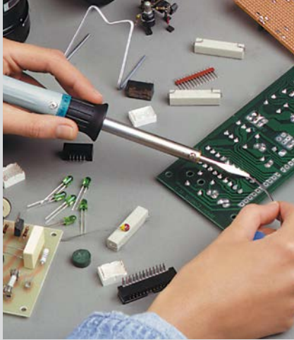
Ersa Universal Soldering Iron – for almost all applications
