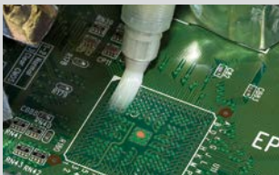
4. Application of flux or solder paste
