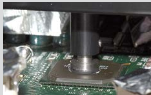
5. Placement of the new or reballed component
