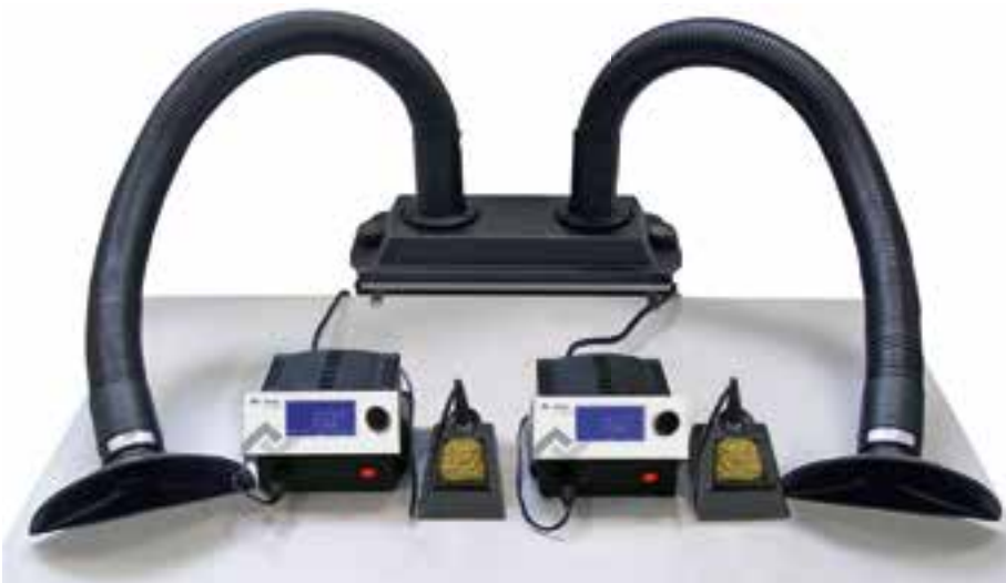
i-CON C soldering stations with EA 110 plus i solder fume extraction: intelligent filter unit control by means of soldering stations' standby function – filter unit is started as soon as one of the soldering stations is operated
