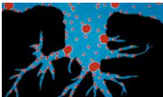
Activated carbon absorbs dangerous gas molecules
